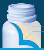
Barrier material Bonding agent Exterior wall HDPE
