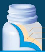
Barrier material Bonding agent Exterior wall HDPE
